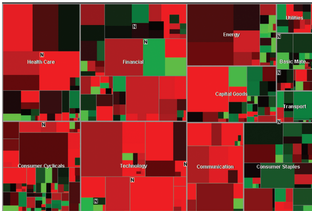
Figure 4.29 A color sequence with black representing zero. Increasing positive values are shown by increasing amounts of red. Increasing negative values are shown by increasing amounts of green. The map itself is a form of treemap (Johnson and Schneiderman, 1991). Courtesy of SmartMoney.com.
