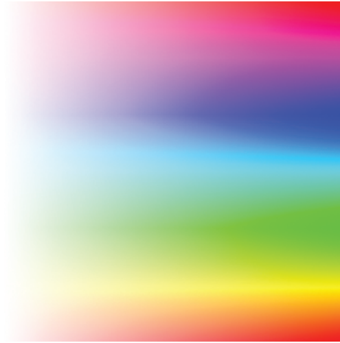
Figure 4.16 This plot shows hue and saturation, based on Smith's transformation (1978) of the monitor primaries.
